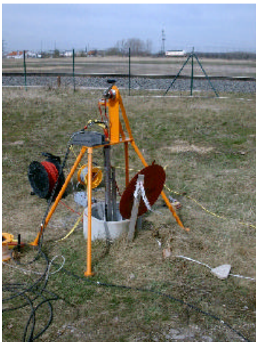
Shear wave source and surface equipment
