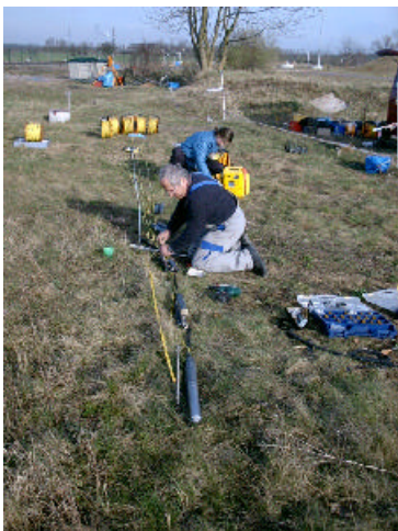
Borehole geophone assembly
