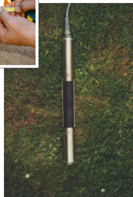
Downhole BGK3 Probe
