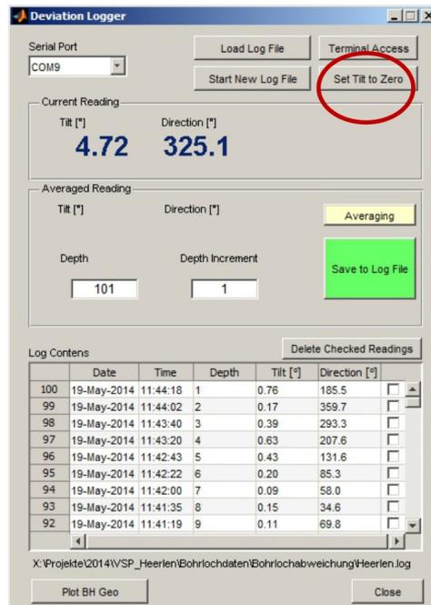
Figure 8: Deviation logger Software and the “Set Tilt to Zero” button
