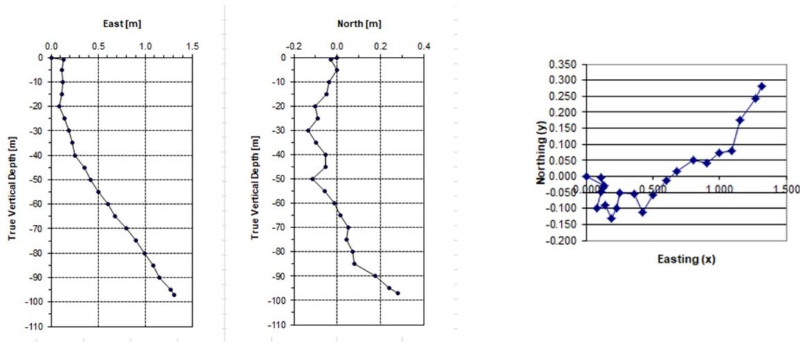
Figure 15: Visualization of borehole deviation
