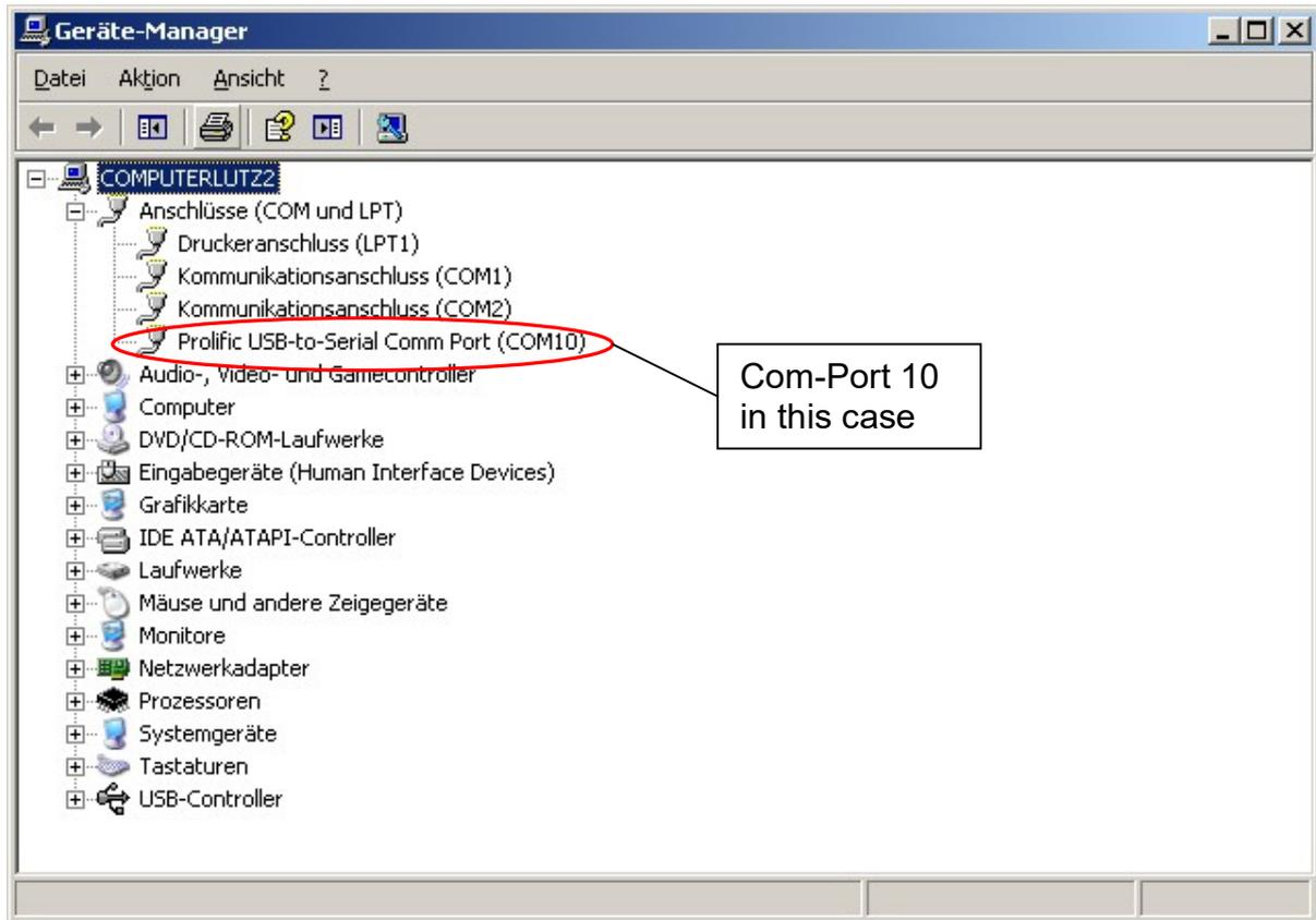
Figure 11: Generated virtual serial interface in Windows Device Manager
