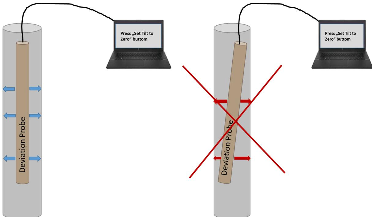
Figure 7: left) correct probe position and right) incorrect probe position for tilt calibration
