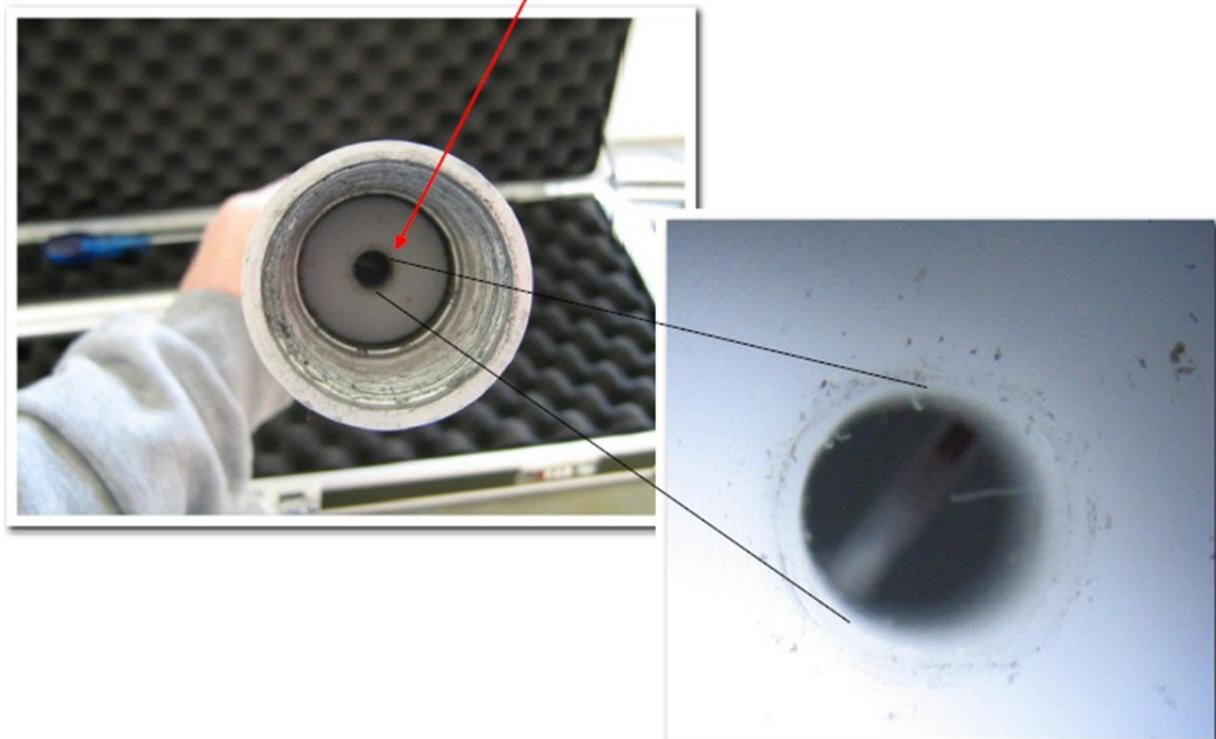
*Figure 6 . Shock indicator is normally white, **red** indicates an external shock*
