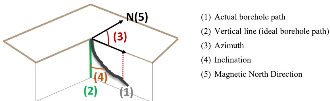
Figure 1: Azimuth and Inclination of a true borehole path
