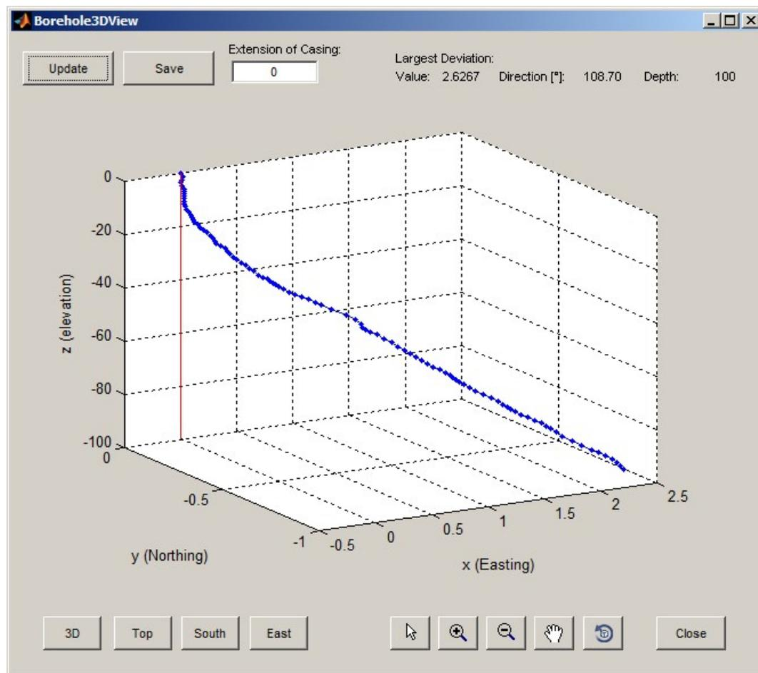
Figure 13: 3D view of the borehole deviation
