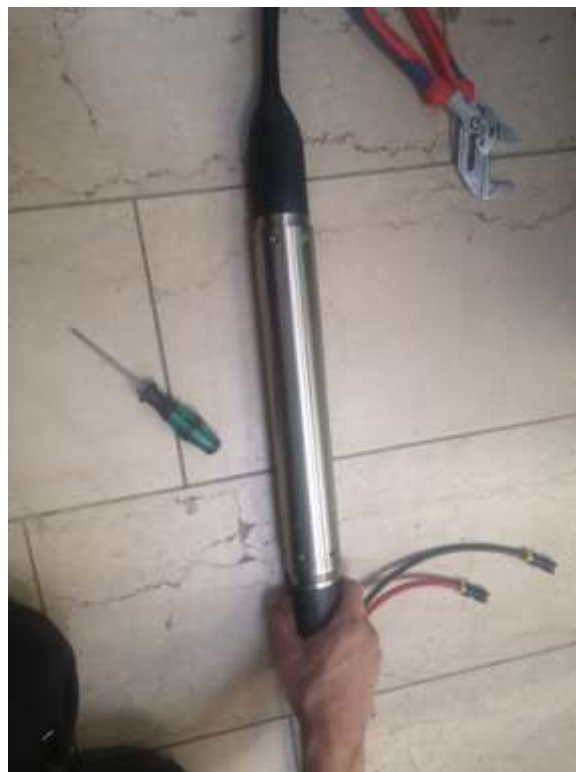
Figure 13: Fix top housing cable and mount all screws
