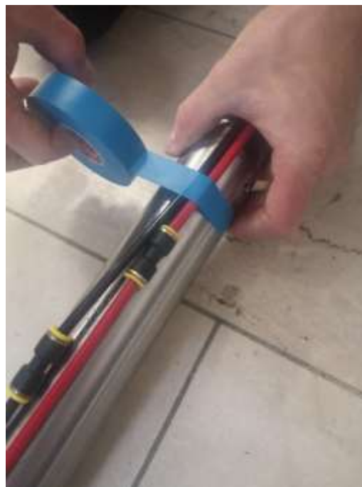
Figure 8: Fix air hoses to cable split using tape
