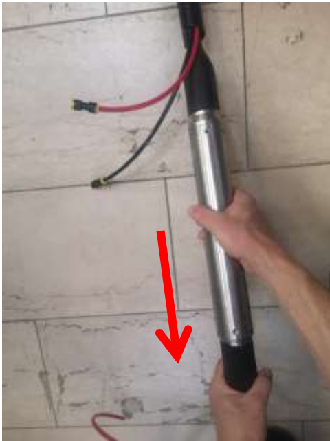
Figure 14: Slide/push steel housing towards bottom cable.
