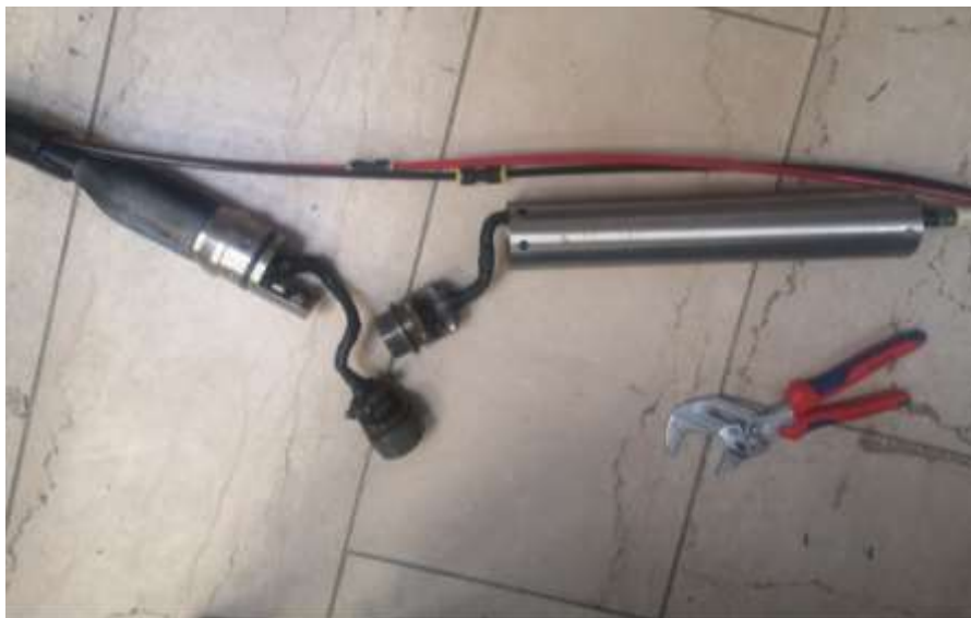
Figure 10: Push the stainless steel housing towards the geophone stations
