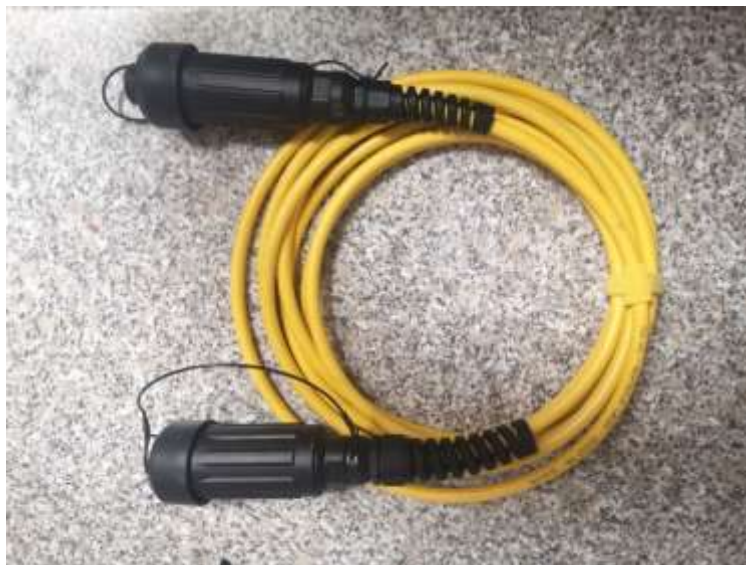
Figure 21: Connecting cable to the seismograph
