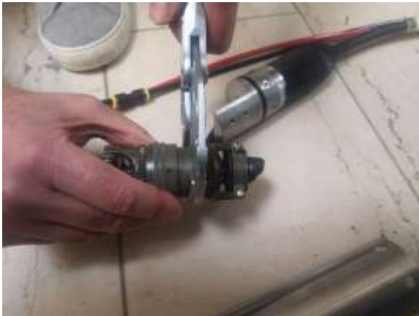
Figure 15: Use pliers to secure to connector. Turn ring on bottom connector counter-clockwise to open.
