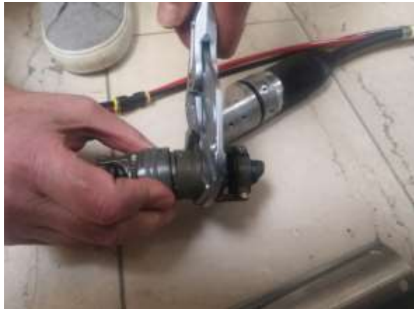
Figure 15: Use pliers to secure to connector. Turn ring on bottom connector counter-clockwise to open.
