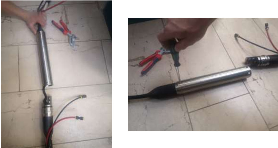
Figure 12: Push housing towards top cable and fix housing at bottom with one screw first
