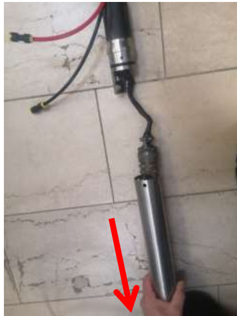
Figure 14: Slide/push steel housing towards bottom cable.
